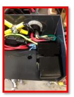
3. Inline fuse. Found inside electrical box. (7.5amp automotive type 2 prong fuse) https://www.youtube.com/watch?v=JZZmYQtybAE replacing fuse
