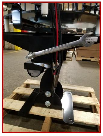
**Step 15** – The pull cord or optional radio release can now be connected to the machine. Pull cord will connect through the yellow- ended cord.
